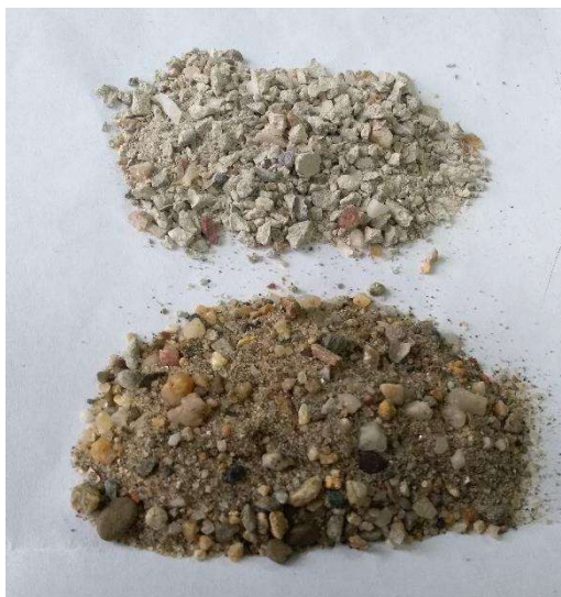
Figure 1. River sand (left) and recycled fine aggregate (right) used in this study
