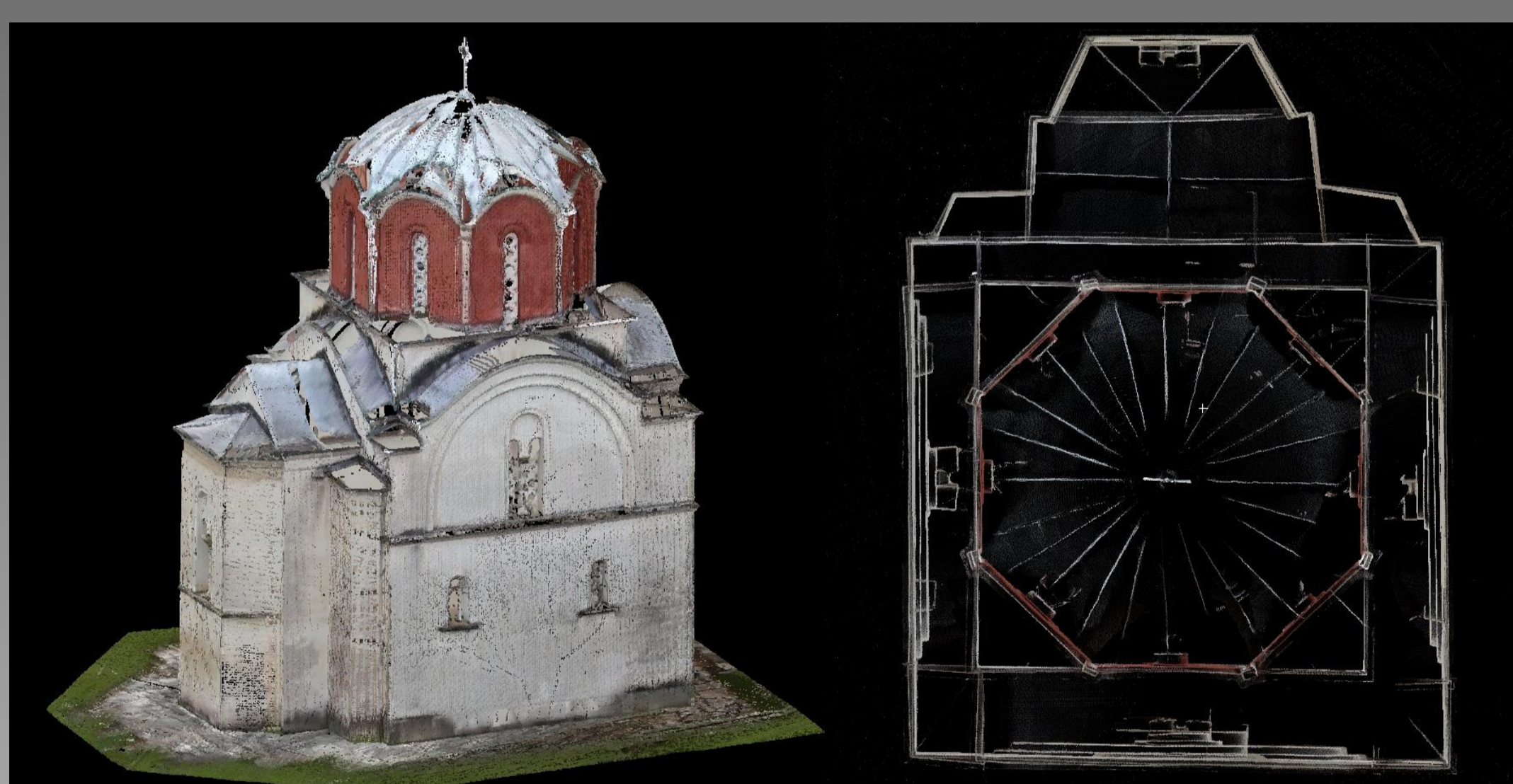
Figure 3 3D (on the left) and 2D (on the right) representations of the church St. Joachim and Ana - point cloud deliverables
