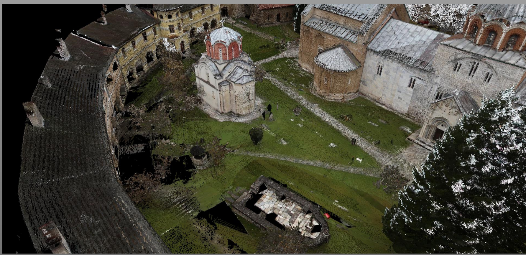
Figure 2 Studenica complex - Photorealistic presentation: part of the scanned area (registered point cloud data)
