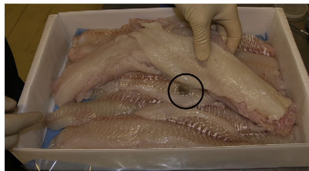
Fig. 1 – Whole haddock fillets in a CP box. Also shown is one of the temperature loggers used for monitoring temperature in between fillets.
