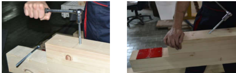
Fig. 6. Preparation of reinforced specimens
