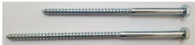
Fig. 3. Screws used as reinforcement
