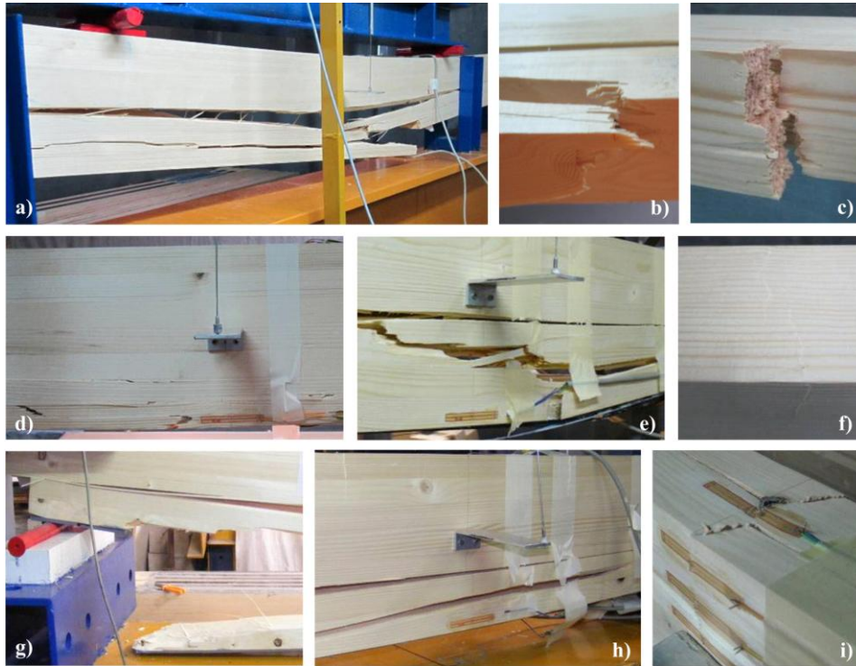
Fig. 3. Beam failure modes
