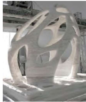
Figure 3. Application of ink printing method by D-Shape. [1]
