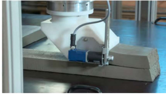
Figure 1. FDM technology for 3D printing of concrete (TU Dresden). [4]
