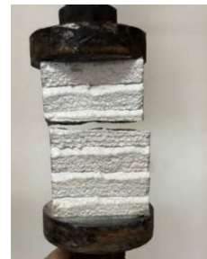
Figure 7. Fracture of sample from series 2 in axial tension test [9]
