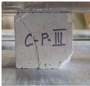
Figure 6. Fracture of sample from series 1 in compressive strength test [9]
