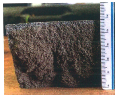
Figure 7: Sample surface after treatment with silver nitrate solution [7].
