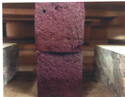
Figure 6: Sample surface after treatment with phenolphthalein solution [7]
