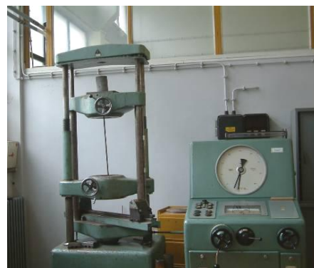
Figure 7. Testing of bond between concrete and reinforcement.
