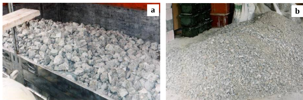
Figure 2. Recycled material after (a) primary and (b) secondary crushing.
