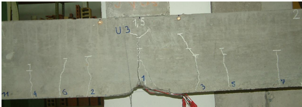
Figure 17. Crack pattern after collapse of beam R50.
