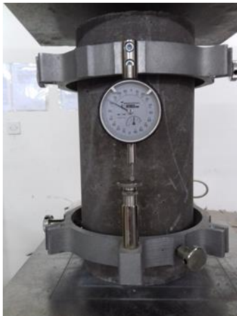
Figure 5. Measurement of the modulus of elasticity of SCC series
