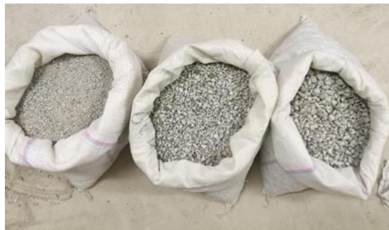
Figure 2. Different sizes of fine and coarse RCA (recycled concrete aggregate)
