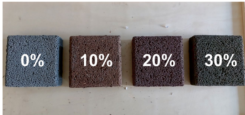
Figure 5. Four investigated pervious paver samples with 0%, 10%, 20% and 30% of solidified wastewater treatment sludge, respectively, going from left to right.
