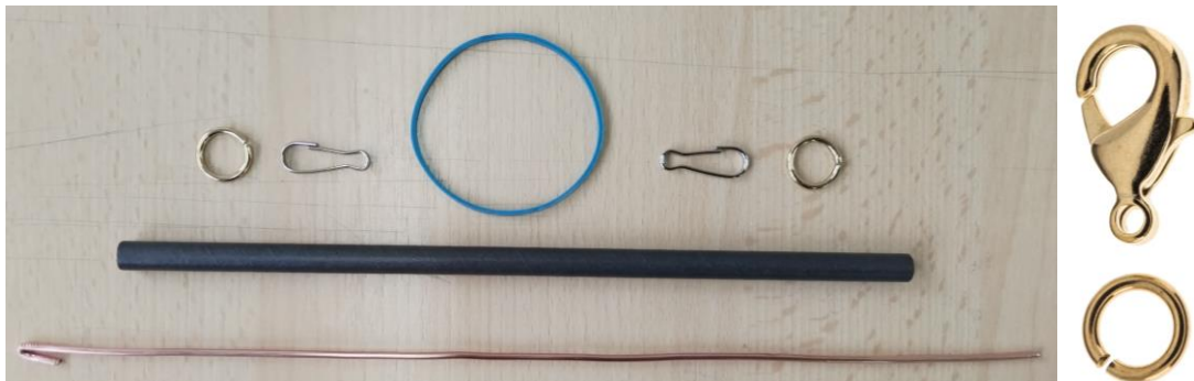
Fig. 3. Basic elements of the platform: (left) ring link, key clasp, rubber band, paper straw for frappe, wire hook for threading the rubber band through the straw, (right): the lobster clasp and the ring link
