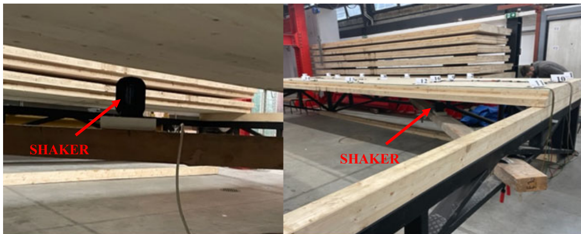
Figure 4. Music shaker and its connection with the supporting frame.
