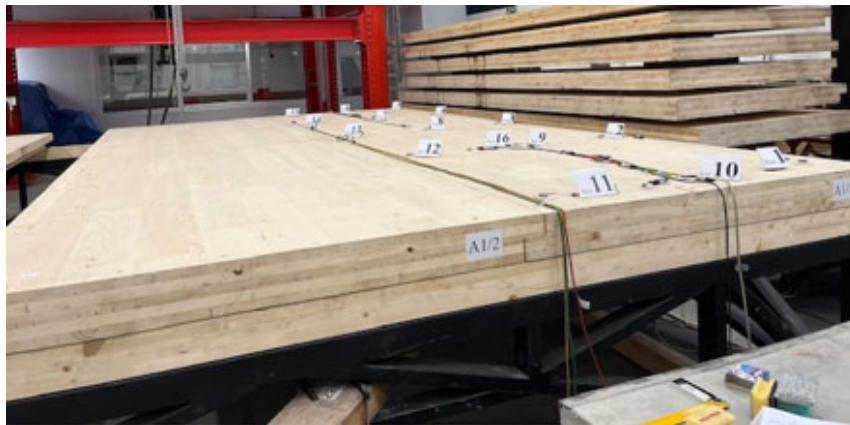
Figure 6. Experimental setup of two-panel CLT floor.
