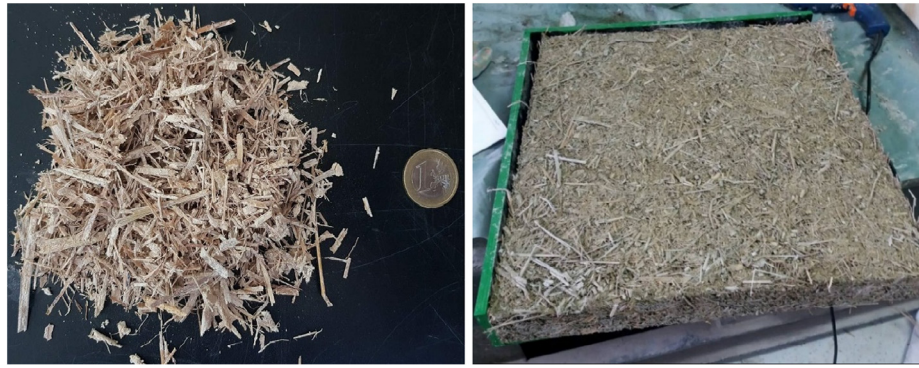
Fig. 1. The used Miscanthus x giganteus bio-fibers and an insulation panel prototype.
