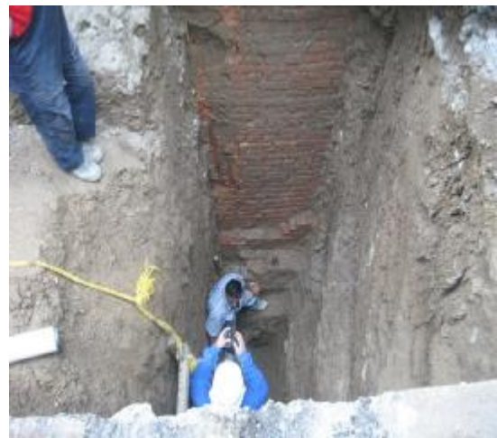
Slika 6. Uzimanje uzorka tla ispod temelja u jami J-1 Figure 6. Sample extracting from trial pit J-1
