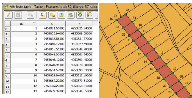
Figure 4: Expropriation zone boundary points layer
