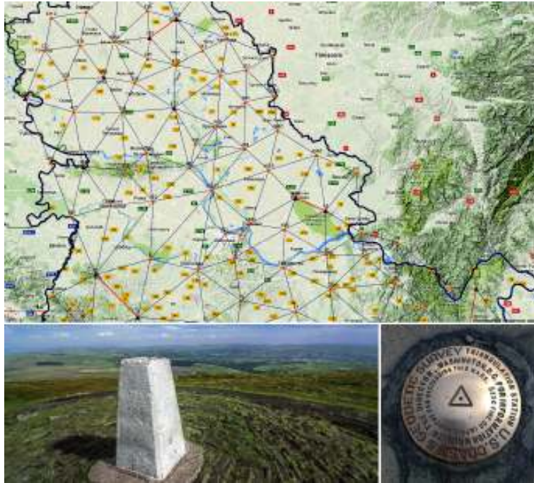
Figure 7. Trigonometric network as a geodetic frame and trigonometric monument with point mark.
