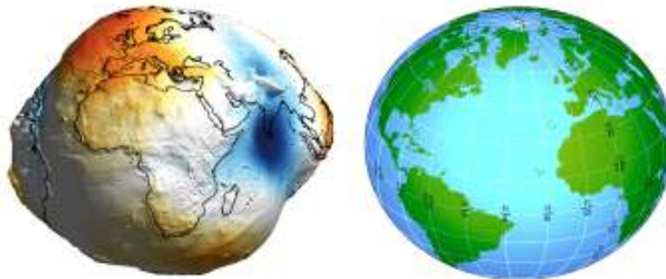
Figure 2. Exaggerated pictures of geoid and flattened ellipsoid
