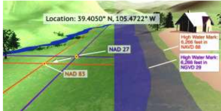
Figure 11. The result of position and height disagreement between two coordinate systems of nor American continent. Horizontal datums NAD27 vs. NAD83 and height datums NGVD29 vs. NAVD88
