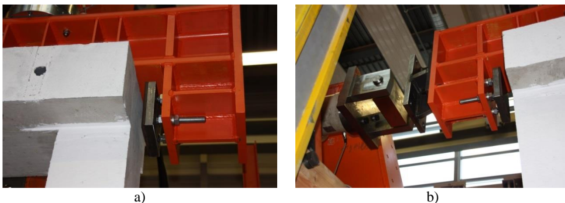
Figure 5.5 a) Elastomeric bearings for reduction of stress concentrations and b) hinges for eliminating vertical force and bending moment at the left end of the load introduction beam
