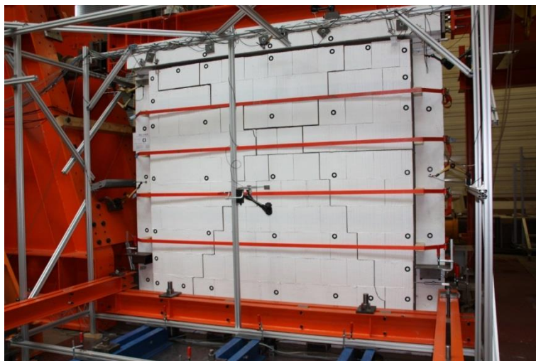
Figure 5.61 Cracks in the wall under maximum out-of-plane load of 6 \text{ kN/m}^2
