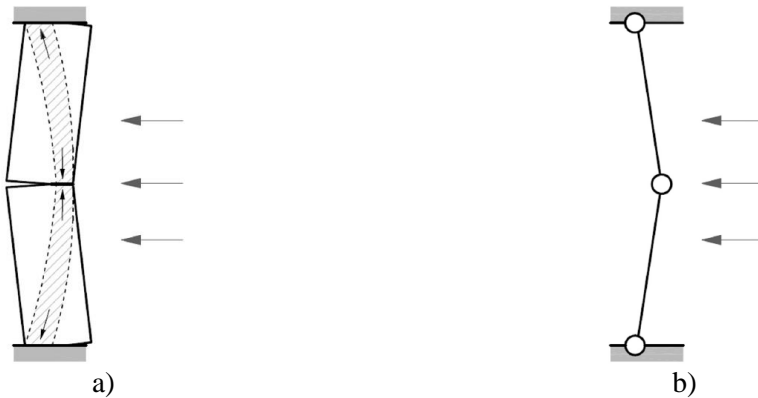
Figure 2.16 Out-of-plane mechanism: a) development of arching mechanism and b) idealized three-pin arch (Asteris et al. 2017)
