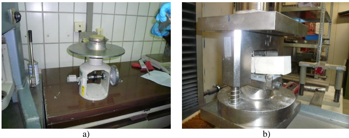
Figure 4.4 a) Determination of slump and b) flexural strength of the mortar (INSYSME, 2017a)
