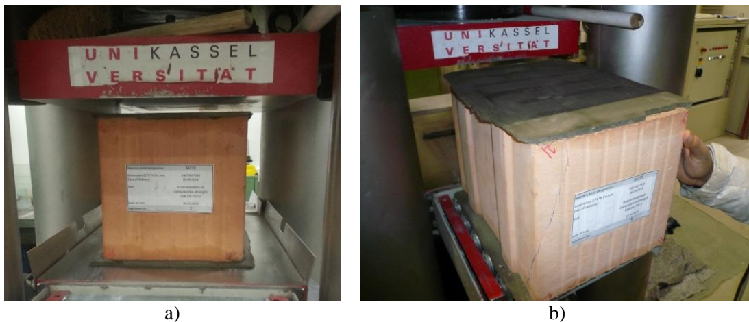
Figure 4.6 a) Determining compressive strength of the masonry units and b) damaged brick after the test
