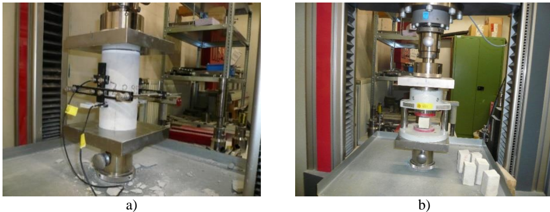
Figure 4.3 a) Determination of elastic modulus and b) compressive strength of the mortar (INSYSME, 2017a)
