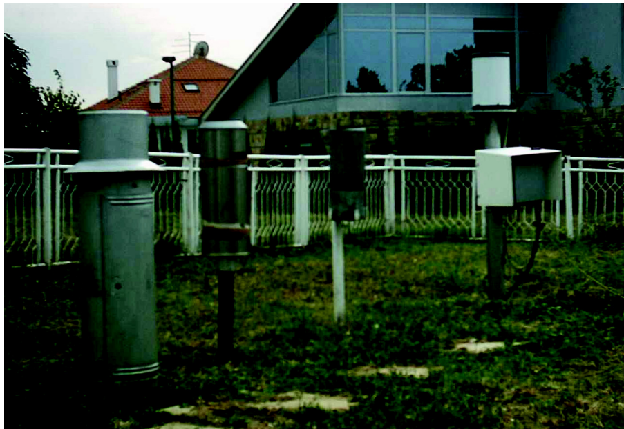
Slika 4. Kišomeri postavljeni u meteorološkom krugu uz zgradu RHMZ. Figure 4. The raingauges mounted at the meteorological station beside the building of the Hydrometeorological Service of Serbia.
