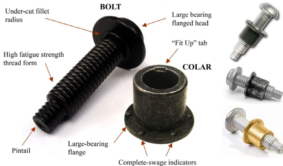
Figure 2. Huck BobTail Bolts consisting of bolt and collar
