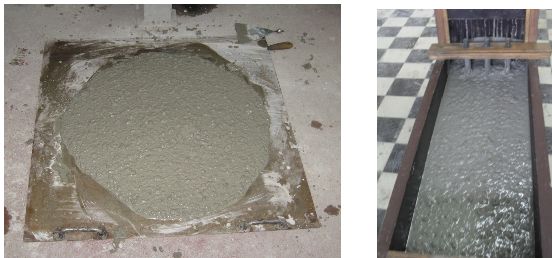
Figure 7: Self Compacting Concrete prepared and tested in laboratory conditions
