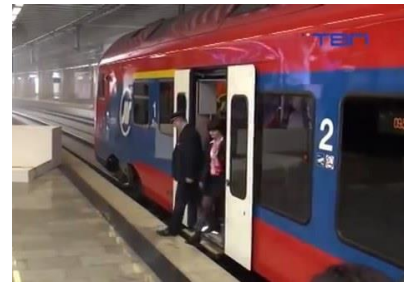
Fig.5. Comfortable and safe access to the platform (platform height 550 mm) from the vehicle
