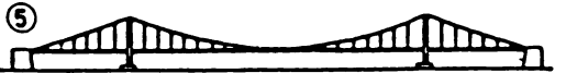
Fig. 4: Earth anchored suspension bridge with the stiffening girder erected from the pylons towards midspan.
