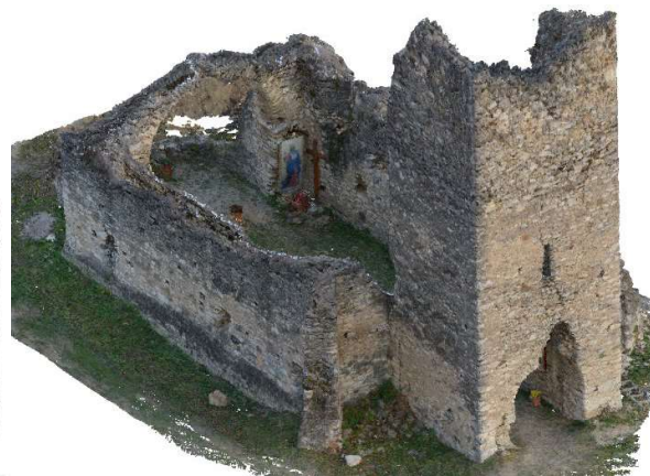
Figure 8: Point cloud obtained by photogrammetric method
