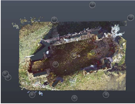
Figure 5: Plan view - the scanner positions
