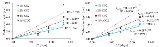
Figure 1. Carbonation depth at CO<sub>2</sub> concentrations of 1%, 2%, 4% and 16% versus time:  $t^{0.5}$  (left) and  $t^{0.75}$  (right)
