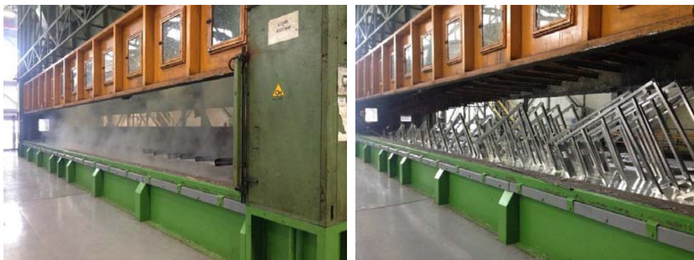
Figure 4 – Hot-dip galvanizing process
