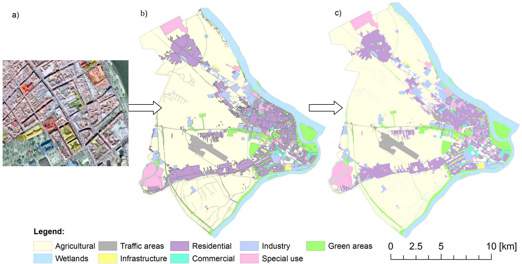
Figure 4.3 a) Digitalization b) Polygons of land use class for year 2001 c) Raster map of land use class for year 2001.
