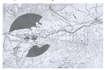
Figure 2 - The Access Surface to the Bled Airport Location (Taken from [4])
