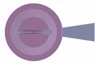
Figure 3. - The imaginary Surfaces of the takeoff-landing track (Top View)
