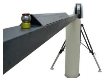
Fig. 2. Laser tracker setup with installed specimen.
