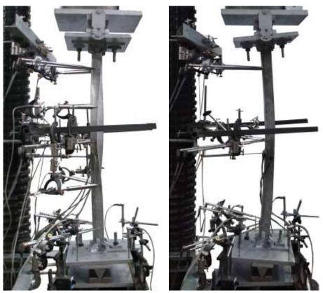
(a) ACF  $80 \times 80 \times 4 - 1000 - 3$  (b) ACF  $80 \times 80 \times 4 - 1000 - 2$ **Fig. 11.** Typical failure modes of specimens in series ACF  $80 \times 80 \times 4 - 1000$ .
