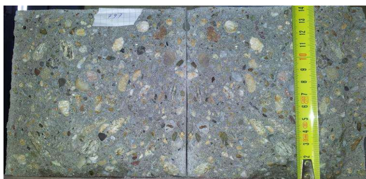
Figure 3 – Maximum water penetration measurement obtained on a sample from SCC-RB series
