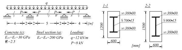
Fig. 1. Continuous composite beam
