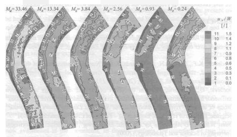
Figure 5. Contour lines showing change in the re-suspension number distribution with respect to the change in the  $M_R$  value at the confluence (d = 0.28 mm)
