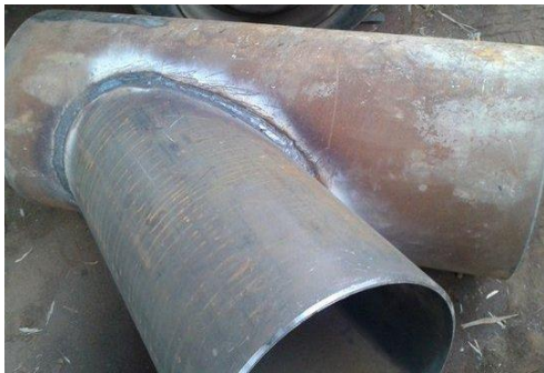
(a) Welding diagram of tee pipe
