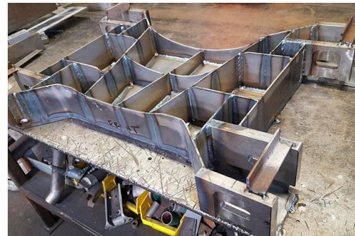
(b) Welding assembly diagram of complex box
