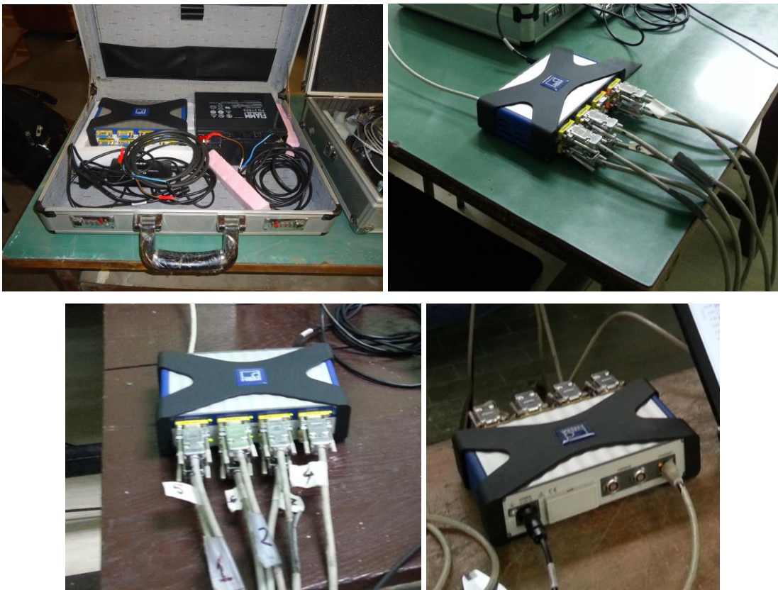
Figure 3.3: Data acquisition device used in the ambient vibration testing
