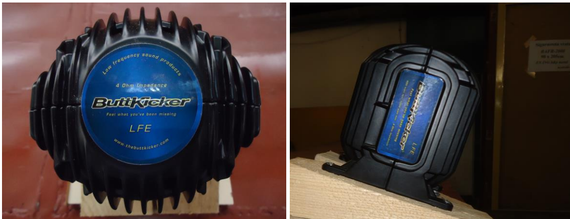
Figure 3.1: Shaker device used in the simulation of ambient vibration testing
