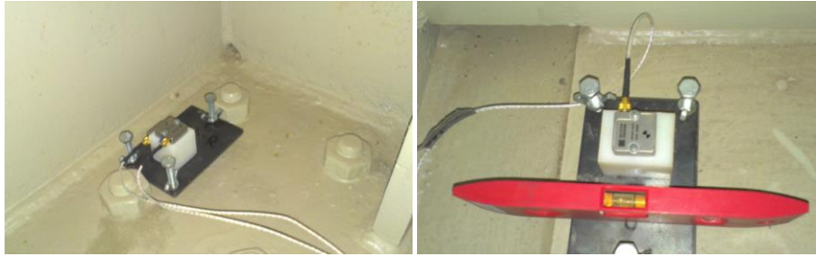
Figure 3.8: Accelerometers inside of left bank approach structure of GAZELA bridge [107]
