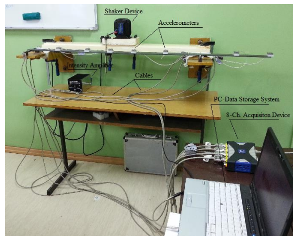
Figure 5.4. Data acquisition system of overhang beam model
