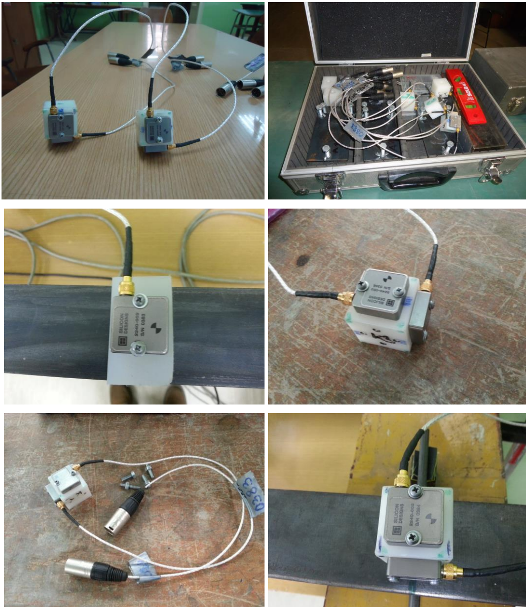
Figure 3.2: Accelerometers used in the ambient vibration testing
