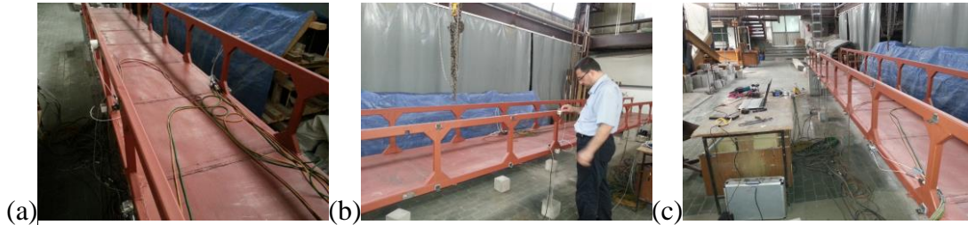
Figure 5.34. Distribution of sets of accelerometer positions along the length of Vierendeel bridge model state without additional masses (a) fourth set, (b) sixth set and (c) eighth set
