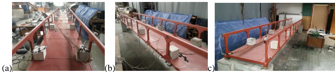
Figure 5.35. Distribution of sets of accelerometer positions along the length of Vierendeel bridge model state with additional masses with additional masses (a) second set, (b) fifth set and (c) tenth set
