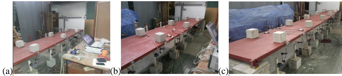
Figure 5.19. Distribution of sets of accelerometer positions along the length of grid bridge model with additional masses (a) first set, (b) third set and (c) fourth set
