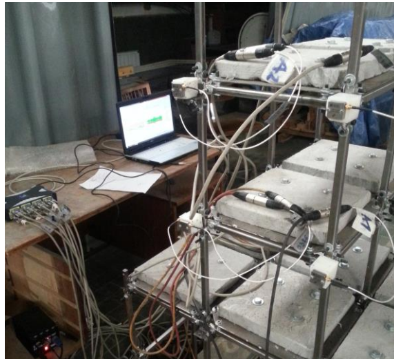
Figure 5.48. Positions of accelerometers of measurement points and movement directions of second set of multi-storey model
