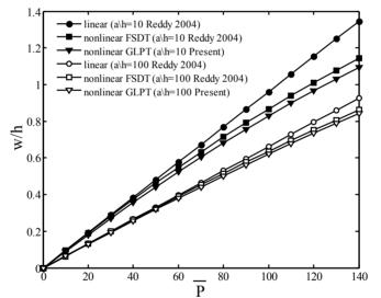
Fig. 3. Nonlinear bending of square simply supported (SS1) orthotropic plate; central displacement versus load parameter.
