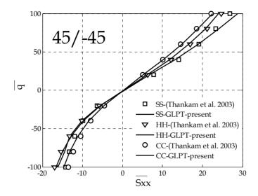
Fig. 7. Nonlinear bending of square angle ply 45/-45 plate with different boundary conditions and a / h = 10; in plane stress  $\overline{S}_{xx}$  versus load parameter.
