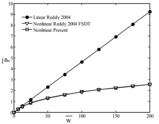
**Fig. 2.** Nonlinear bending of square simply supported (SS1) isotropic plate with a/h = 10; central displacement versus load parameter.
