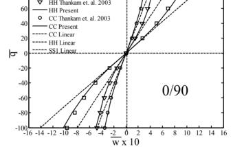
Fig. 4. Nonlinear bending of square cross ply 0/90 plate with different boundary conditions and a / h = 10; central displacement versus load parameter.
