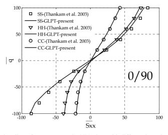
Fig. 6. Nonlinear bending of square cross ply 0/90 plate with different boundary conditions and a / h = 10; in plane stress  $\overline{S}_{xx}$  versus load parameter.
