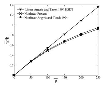
Fig. 8. Nonlinear bending of square simply supported (SS1) general quasi-isotropic (0/45/-45/90)s laminated plate with a / h = 10; central displacement versus load parameter
