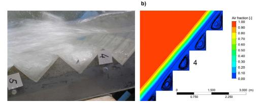
Figure 5. Air entrainment at the stepped spillway obtained by: a) scale-model, b) numerical model. The recirculating flow in the triangular cavity, formed by the steps, was observed on the scale model as well as the air entrained in the cavity. The numerical model was able to reproduce the recirculating flow pattern in the cavity (see the streamlines). Modelling of air water mixing was restricted to the free surface zone, but was not reproduced within the cavity itself.
