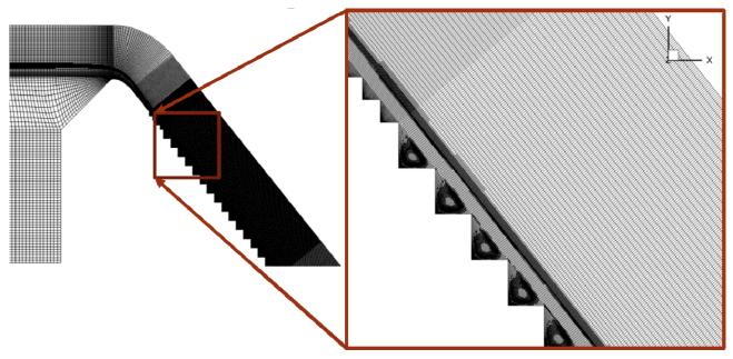
Figure 3. Computational mesh for the prototype stepped spillway. Initial mesh was refined in the areas of steep velocity gradients, intense air-water mixing near the free-surface as well as in the triangular cavities where rotational flow conditions were expected. Rough mesh was used upstream of the weir as the velocities were two to three orders of magnitude smaller than the ones along the spillway.
