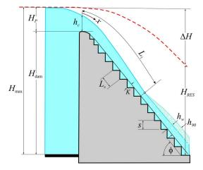
Figure 2. Cross-section of the typical stepped spillway dam with quantities used in the empirical equations [14]
