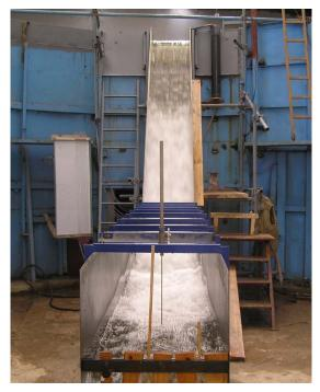
Figure 1. Scale model of the section of the weir with the stepped spillway of the Bogovina dam [14, 20]
