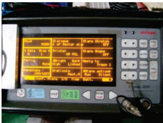
Figure 4 The device Phasec 2200 for rail testing using the EC
