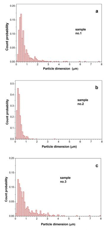
**Fig. 5.** Particle size distribution based on SEM analysis a) sample no.1, b) sample no.2 and c) sample no.3.
