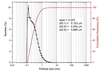
Fig. 1. Particle size distribution of BGO powder.
