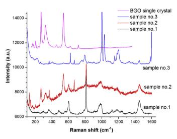
Fig. 7. Raman spectra of BGO single crystal and composite samples.
