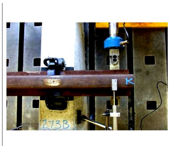
Slika 2. Postavka ispitivanja za određivanje otpora zaokretanju šine i primer dijagrama otpora zaokretanju šine Figure 2. Test arrangement for determination of torsional resistance and an example of torsional resistance diagram
