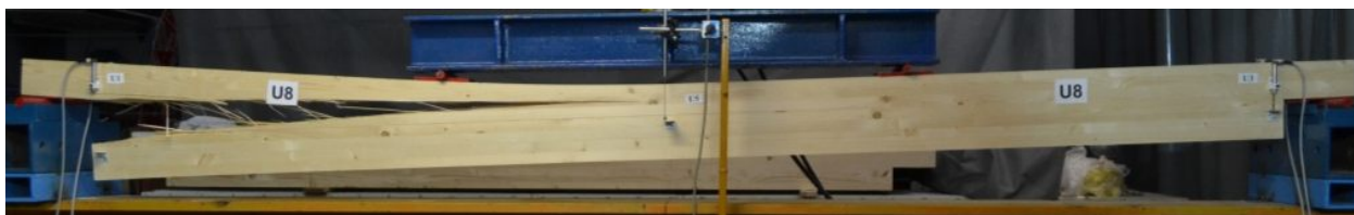
Slika 9. Tipični mehanizam loma grede Serije U Figure 9. Typical failure mechanism of Series U beams
