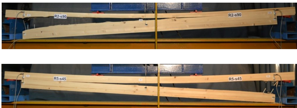
Slika 10. Tipični mehanizam loma ojačanih greda – Serija R Figure 10. Typical failure mechanism of reinforced beams – Series R
